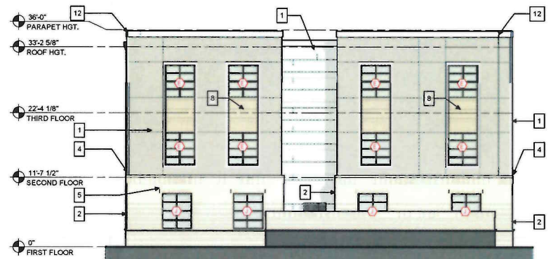
4 PHASE 5A - NORTH ST ELEVATION 3/32" = 1'-0"
