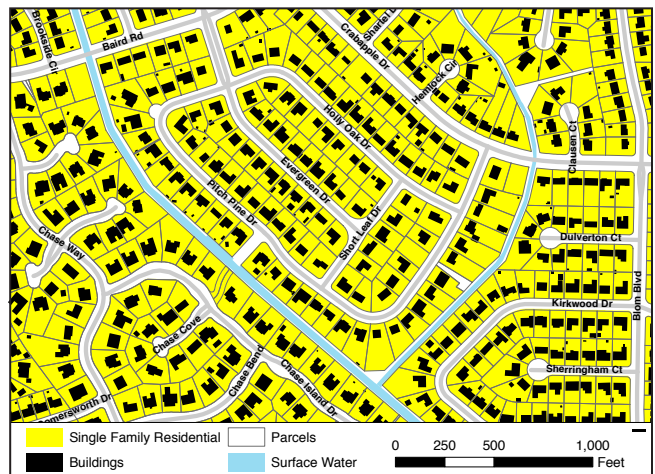
Curved roadways, larger blocks and multiple cul-de-sacs typical of postwar suburban development
