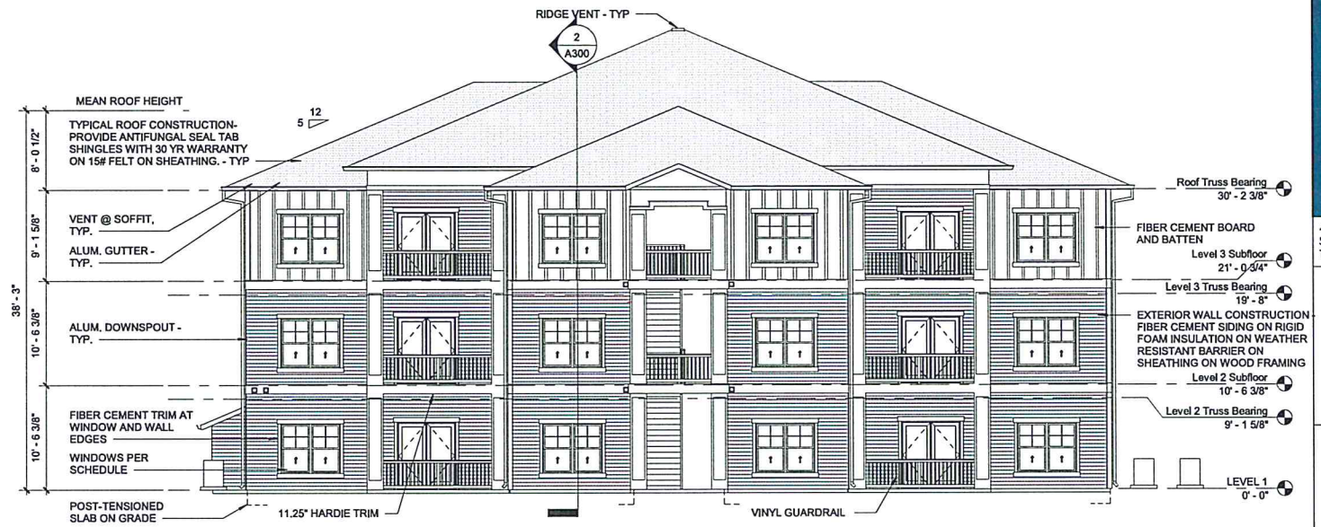
4 BACK ELEVATION - BLDG B 1/8" = 1'-0"
