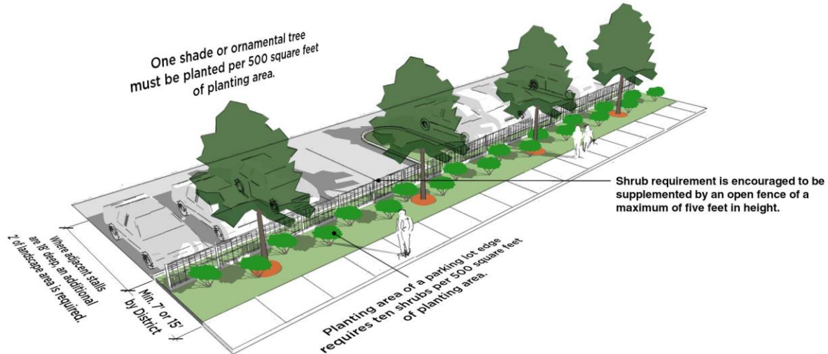
FIGURE 10-3: PARKING LOT PERIMETER LANDSCAPE
