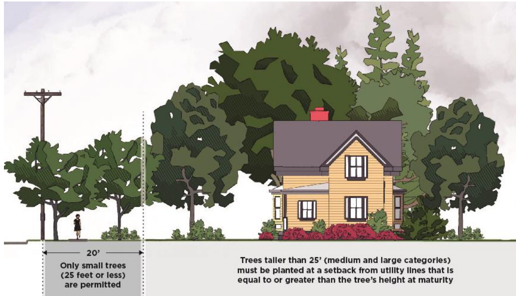
FIGURE 10-1: OVERHEAD UTILITY PLANTING ZONES
